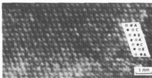
Figure 3. HREM image along the [010] zone axis showing a local 6R martensite in step-quenched Cu-17.4 at.% Zn-13.0 at.% Al alloy.
